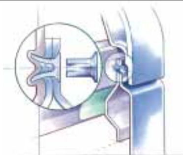
Aircraft-style, self-piercing fasteners are stronger and produce a smooth outer skin for an extraordinary finish.
